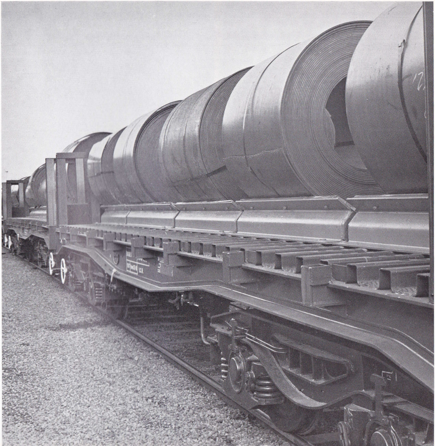
Right: Coiled plate loaded on 100-tonne rail wagons, ready for despatch
