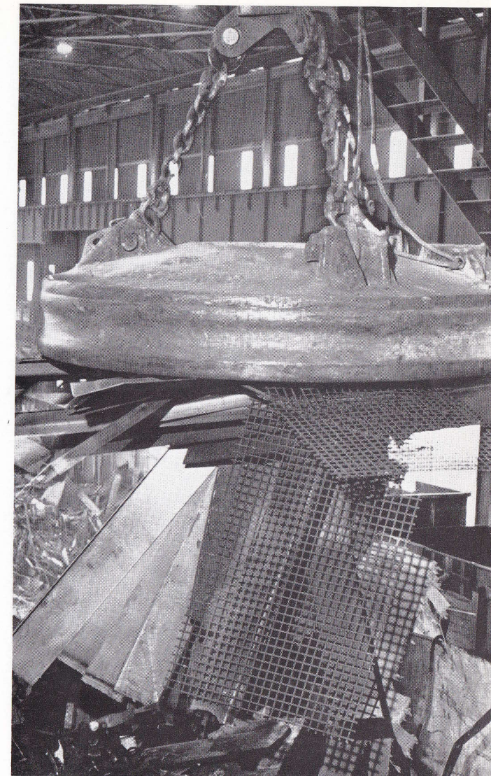
Scrap handling at the electric arc plant, Cleveland
