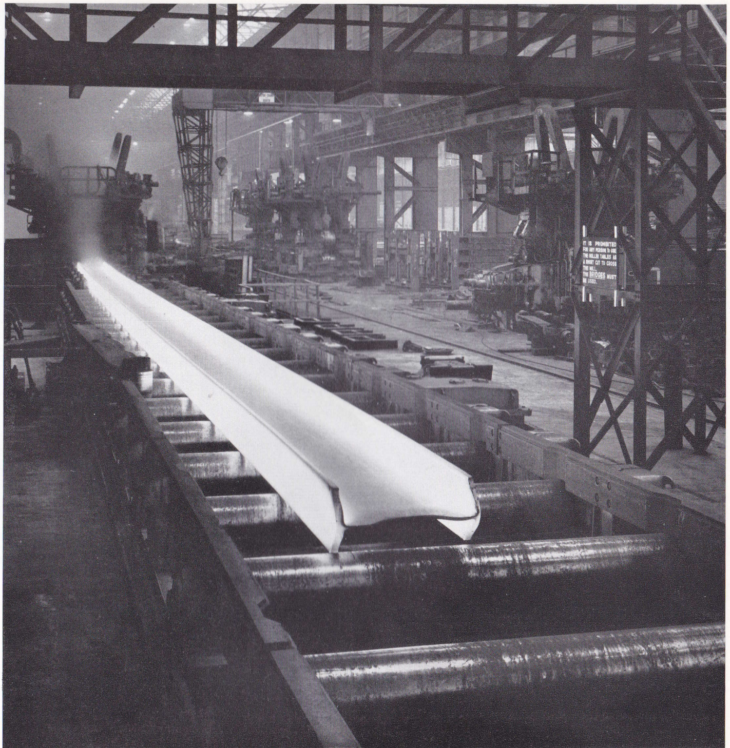
The blooming mill and right the rolling of large universal beams at the Lackenby beam mill
