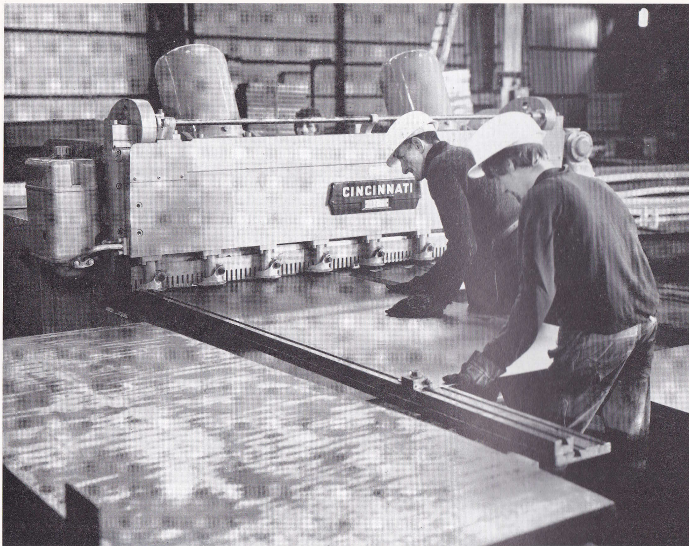
Shearing light plate in readiness for sheet metal fabrication at Ayrton
