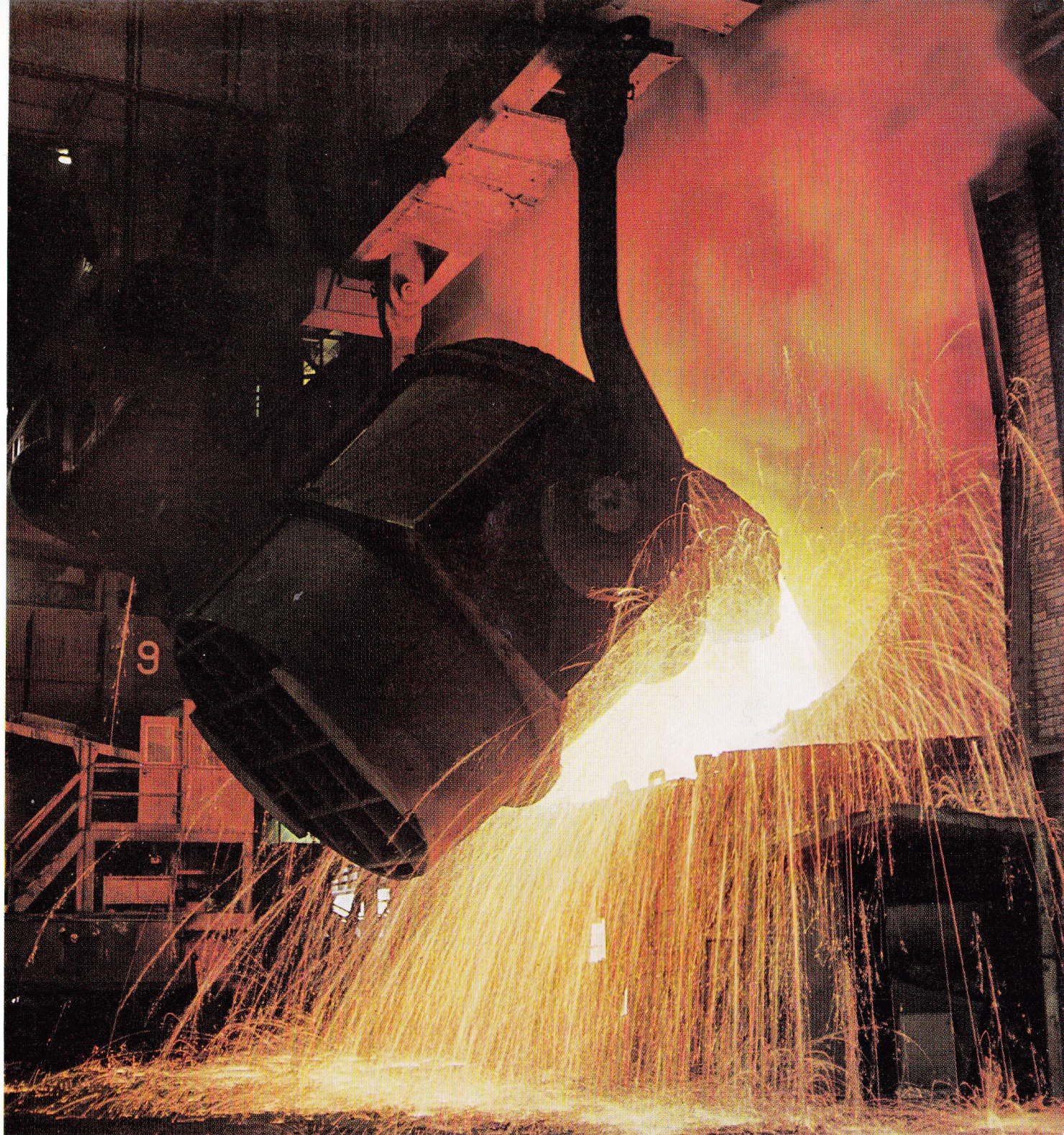
Hot metal charging at the Lackenby BOS plant
