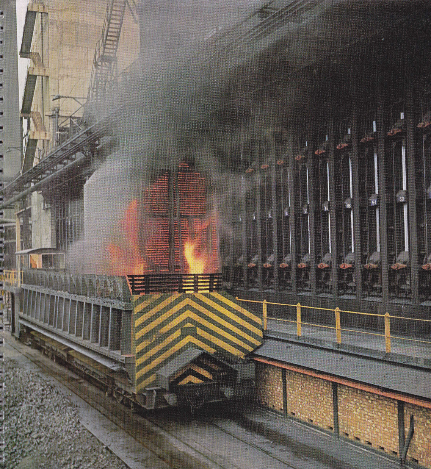
Pushing coke at the South Bank coke ovens
