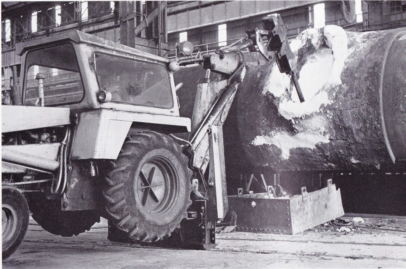
Skulling of torpedo ladles at Cleveland Works
